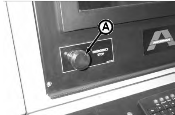
E-Stop on Control Container Console
