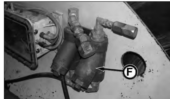
Strainer Shown In Trailing Dolly
