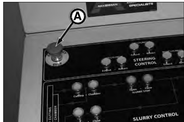
E-Stop on Control Container Console
