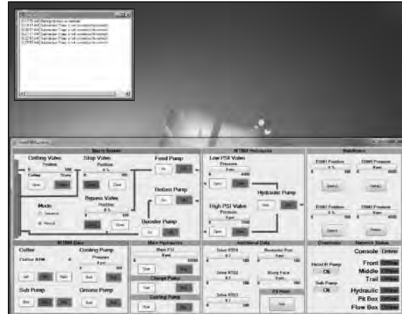
Log Message and MTBM Control Screens
