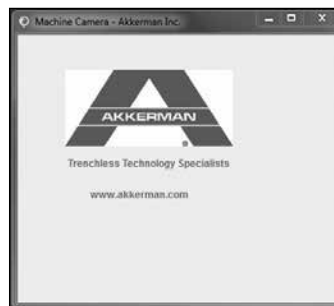
MTBM Camera Screen With No MTBM Ethernet Connection
