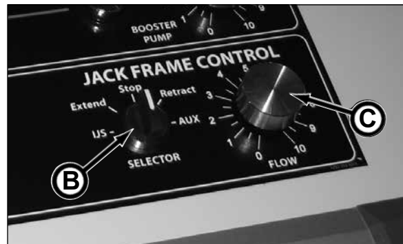
Jacking Hydraulics Start Up On MTBM Control Screen
