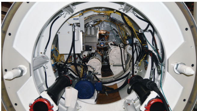
Figure 14. Propulsion or Jacking and Lubrication Cans exert even jacking force for smooth advancement and house lubrication feed valves for the MTBM.
