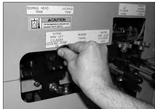
Extending Ram Lift Cylinders SN F20400F-01 Shown
