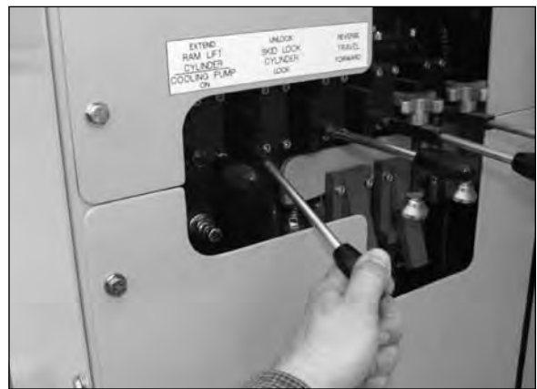
Locking Skid Lock Blocks SN F20400F-02 & After Shown
