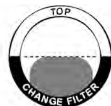
Filter Needs Service
