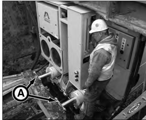
Extending Main Ram Jacking Cylinders
