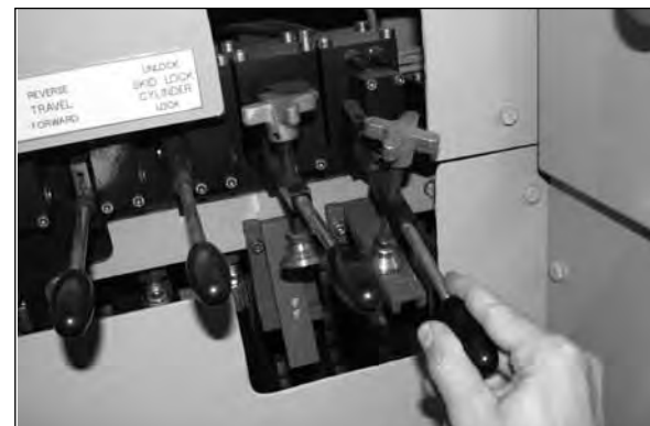
Extending Main Ram Jacking Cylinders
