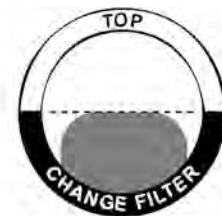
Filter Needs Service
