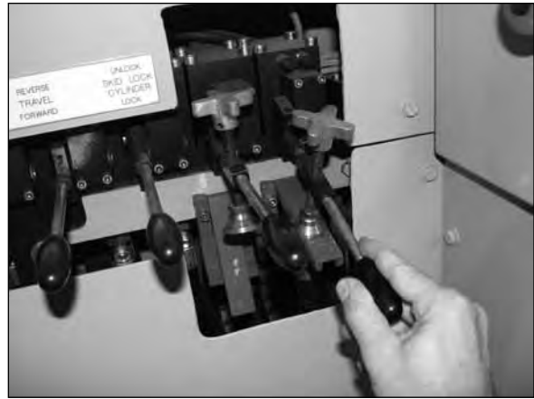
Extending Main Ram Jacking Cylinders
