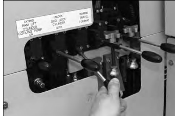
Pump Unit Forward Travel Control SN F20400F-02 & After Shown
