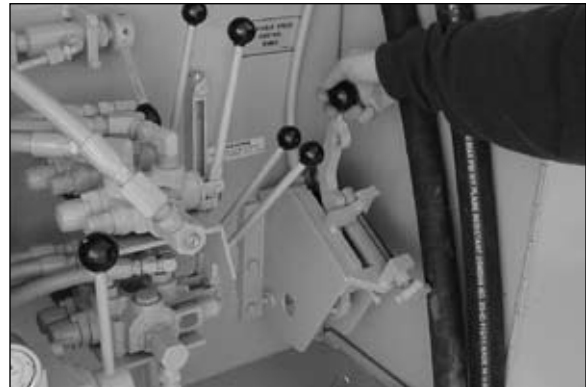
5000 Pump Unit - Cable Stroker Control
