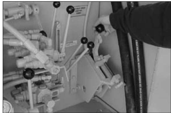
5000 Pump Unit - Cable Stroker Control
