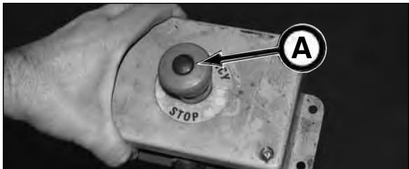
Remote E-Stop on 5000 Series II Pump Unit
