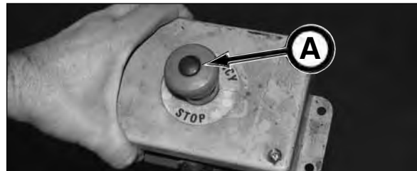
Remote E-Stop on 5000 Series II Pump Unit
