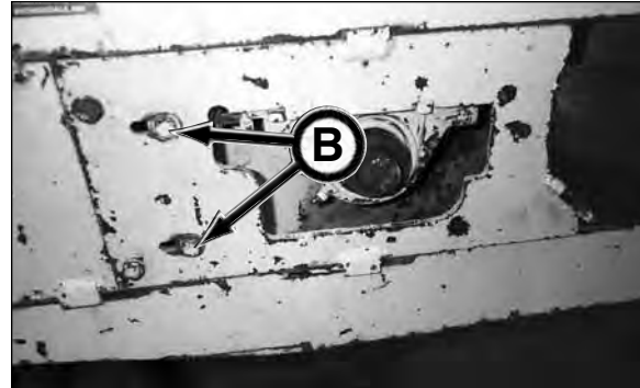
Internal Drive Roller Scraper Adjustment
