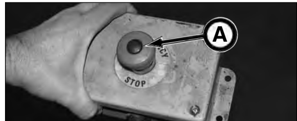
Remote E-Stop on 5000 Series II Pump Unit
