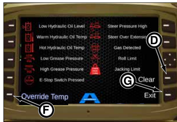
Active Alarm Screen With High Oil Temp Fault
