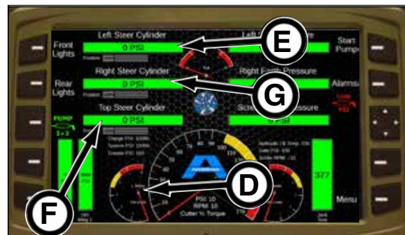
System Pressure (Load Sense) (D) Steering Cylinder Pressure - Left (E) Steering Cylinder Pressure - Top (F) Steering Cylinder Pressure - Right (G)
