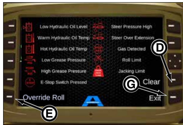
Active Alarm Screen With Roll Limit Fault
