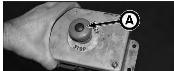
Remote E-Stop on 5000 Series II Pump Unit
