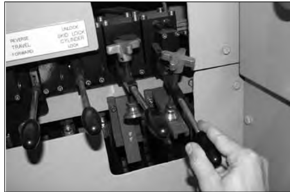
Extending Main Ram Jacking Cylinders
