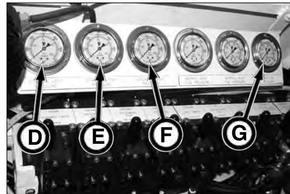
Steering Cylinder Pressure - Left (D) Steering Cylinder Pressure - Top (E) Steering Cylinder Pressure - Right (F) System Pressure (G)
