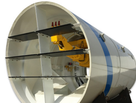
Figure 5. The EBS matches the diameter of the pipe and an interior mounted backhoe excavator removes spoil which is transported from the conveyor to the haul unit system.
