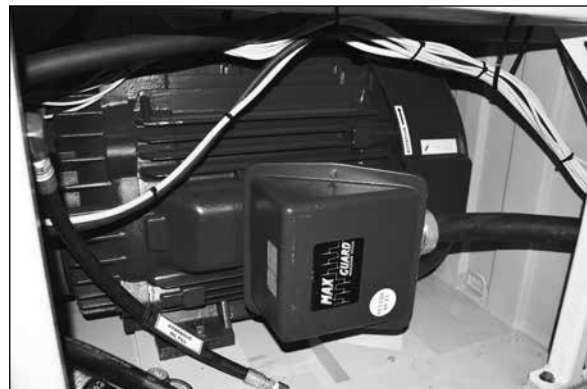
166 HP Electric Drive Motor
