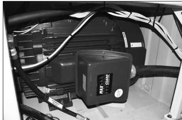
200 HP Electric Drive Motor
