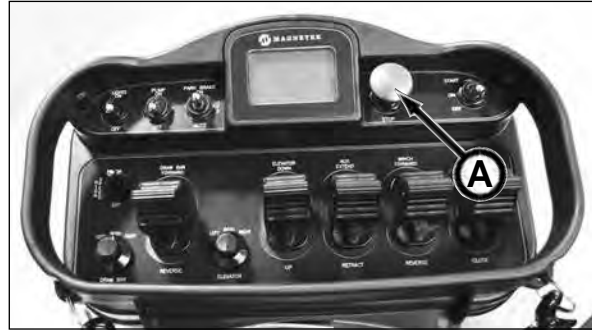
Sliplining Wireless Remote Pendant E-Stop Button
